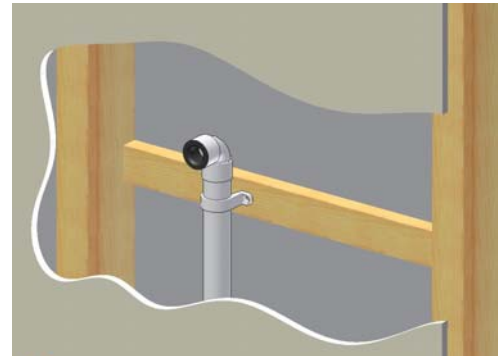
Figure 15: Fit Vertical discharge condensate pipe
