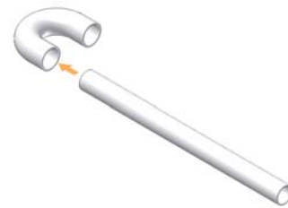
Figure 16: Fit bend to 22mm pipe.
