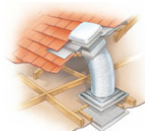
A typical ducted roof installation
