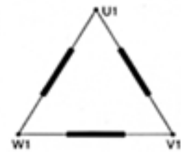
Collegamento Δ Connection Δ Connection Δ
