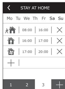
To disable the air handling unit, you can set the STANDBY mode, or when setting the program's events just make a break at the times when the unit must not operate.
