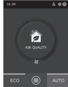
In the “Air Quality” settings menu item, the user can set the maintained air quality or humidity value, as well as the maintained temperature, and can deactivate the electric heater in the unit, if necessary.
