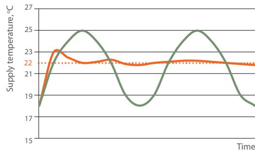
Variable speed compressors are designed in RHP Pro units. The major benefit of this type of compressor is its flexibility. The rotation speed of the compressor varies, as the result less energy is used and the minor temperature changes occur in the premises.
