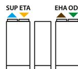
▶ ODA – outdoor intake    ▶ SUP – supply air    ▶ ETA – extract indoor    ▶ EHA – exhaust air
