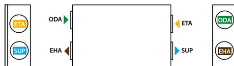
▶ ODA – outdoor intake    ▶ SUP – supply air    ▶ ETA – extract indoor    ▶ EHA – exhaust air
